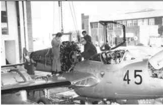
No 25 SQD Fitters are here installing a Rolls-Royce Goblin engine into a 2FTS Vampire in '68.
