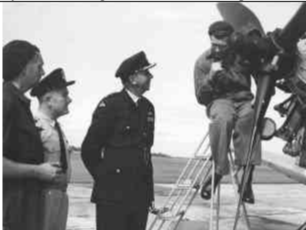
No 25 SQD Fitters are here installing a Rolls-Royce Goblin engine into a 2FTS Vampire in '68.
